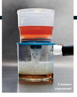
a spinning magnet to stir and gently warm the broth while the pump reduces the air pressure inside the flask. As the pressure drops, the boiling point of the liquid falls as well; the goal is to sustain a mild, low-temperature boil.
